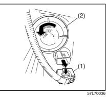
2) To create the space necessary for performing the steps that follow, disconnect the coupler (1) by pressing the claw.
